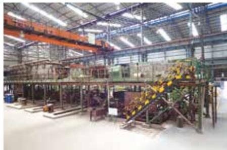
The Otto Junker degreasing, annealing and pickling (DAP) line
